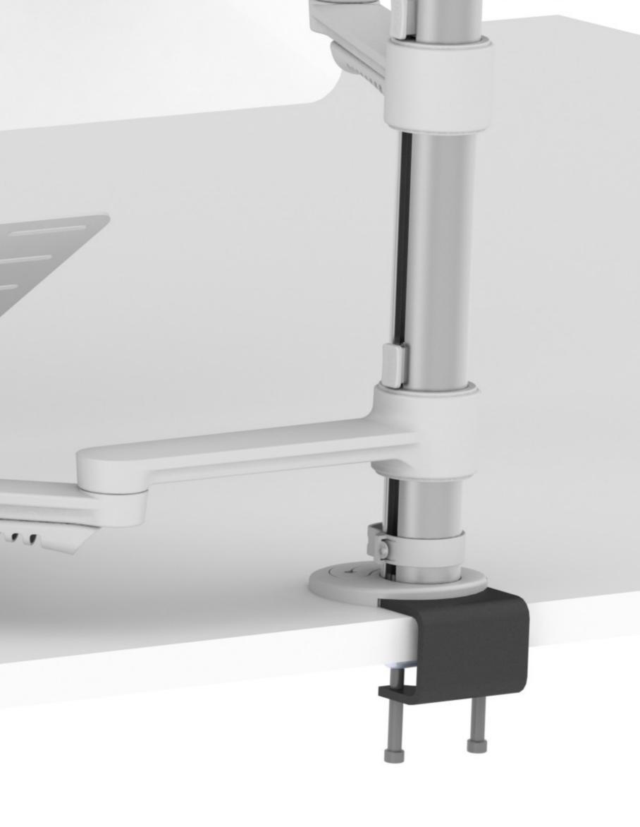
360 degree rotation around the posts – enables the post to be used from both sides of the workstation if required. C.ME can support a maximum 8kg weight per arm. Post height for standard is 430mm allowing for 330mm adjustment. Post height for long posts is 740mm allowing for 695mm adjustment
