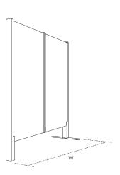
Width narrow screen (W) Width wide screen (W) Height (H) 1000 / 1200mm 1400 / 1600 / 1800mm 1400 / 1600 / 1800mm
